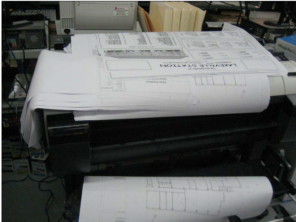
Three jobs comprising three different page sizes sorted on top of the Canon imagePROGRAF iPF765 immediately after removal from stacker basket
