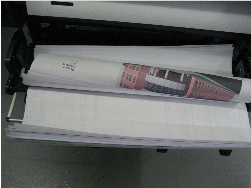
First 30 of 48 pages beginning to curl in Canon imagePROGRAF iPF765 stacker basket
