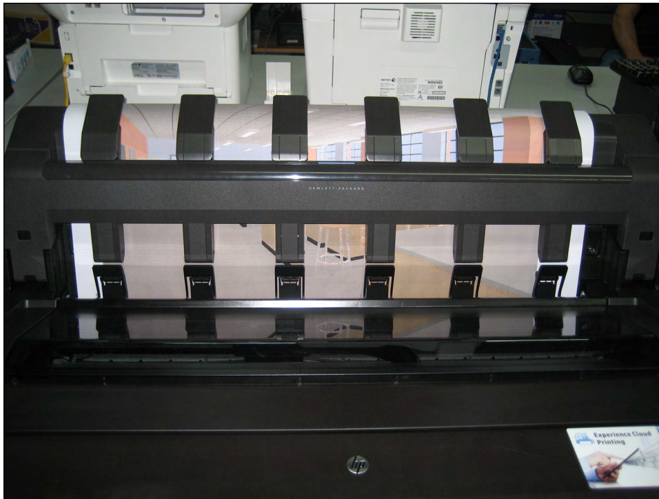
HP Designjet T920 with 48 pages, including three different page sizes in the stacker
